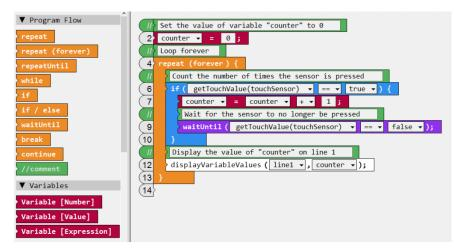
Fig. 7 Screenshot of RobotC Graphical DSL's click-and-drag command blocks [79].
