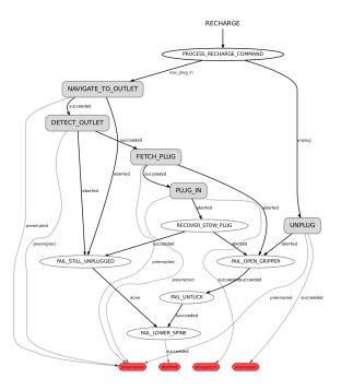
Fig. 2 State machine for a mission that instructs the PR2 robot to charge itself at a standard outlet.
