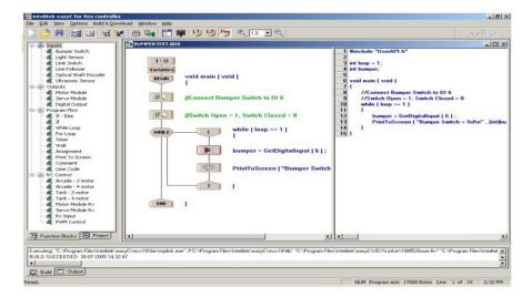
Fig. 3 A screenshot showing EasyC DSL: first column presents the language feature abstractions, second column is the active mission being specified while the last column shows the generated code
