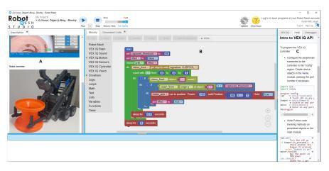
**Fig. 1** Screenshot of the Robot Mesh Studio IDE [78] with three panes. Pane A provides an rich-text description of the mission, Pane B the actual mission expressed in a DSL with Blockly syntax, and Pane C shows help text or alternatively the debugger or an overview on the current robot configuration.
