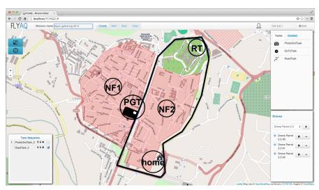
Fig. 5 Specifying a mission for a drone to hover in given space while avoiding no-fly zones [26].
