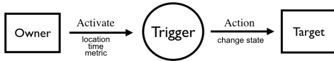
Fig. 5. GeoScenario Trigger. When the owner activates a trigger, an action is executed on the target. The trigger can be activated when the owner reaches the trigger node location, when the Scenario reaches a certain time t , or when a metric between two agents reaches a certain value x .
