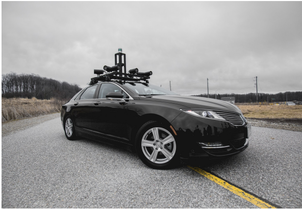
Fig. 7. Autonomoose research platform. Lincoln MKZ Hybrid modified to autonomous drive-by-wire operation and a suite of lidar, cameras, inertial and vision sensors
